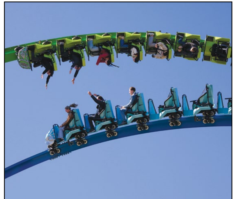
YoY features two tracks, one with inversions and one without. Interaction is what makes YoY different than all other coasters at the park. COURTESY WALIBI HOLLAND
