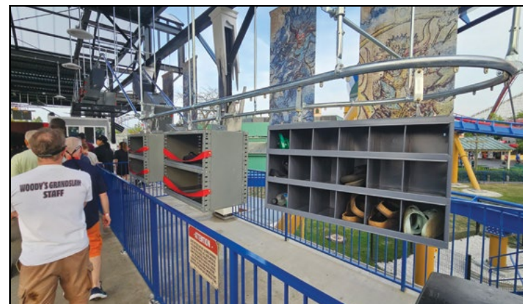
A loose-items mechanism takes loose articles from one side of the loading side of the station to the unloading side. AT/TIM BALDWIN
