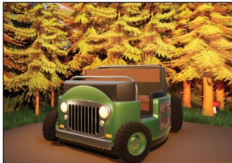
The Rogue Rides vehicle can accommodate five with separated seating (above left) or six passengers (above right) with bench seating. Rogue Rides vehicles are omnidirectional and feature onboard sound and lighting. COURTESY BOLDMOVE NATION
