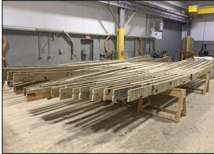
The Gravity Group engineers the track offsite (above left) to precise specifications and then transports the track to the park ready to install. Mighty Canadian Minebuster (above right) is one of the park's original rides, and was the tallest roller coaster at the park when it opened in 1981. COURTESY THE GRAVITY GROUP; AT/TIM BALDWIN
