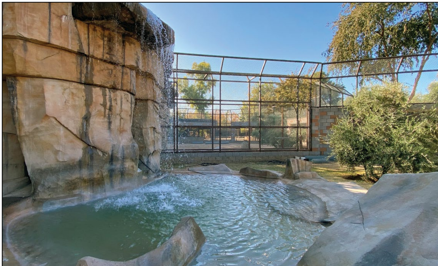
The Wildlife World Zoo's new tiger exhibit is expected to open this spring and features two mirror image habitats with common sleeping rooms behind a waterfall (above). A stainless steel woven cable, oxidized black has been used for the netting. The panels, from A-to-Z Netting in Tucson, Arizona, were chosen for their exceptional strength and durability and to enhance visibility. AT/GARY SLADE
