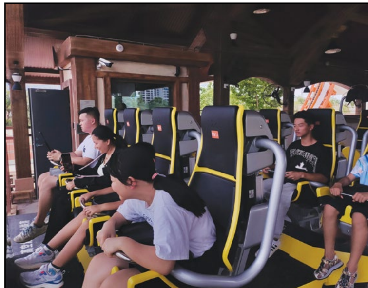
The coaster features four inversions (above). The overhead lap bars of Zamperla's Lightning train allows for comfortable upper-body freedom (below). COURTESY ZAMPERLA
