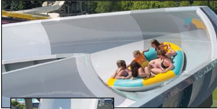
As riders gain speed in the open channel, the raft banks along the side walls (above). A sudden drop accelerates the rafts so they can climb the near-vertical wall (left). COURTESY CANADA'S WONDERLAND
