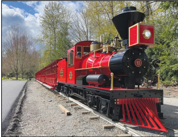
Above left is the Swannee River Railroad new 24-inch gauge, SR24-Steam Outline (located at Remlinger Farms of Carnation, Washington), which features a 75 horsepower and four cylinder turbo-charged Kohler Diesel with six coaches. The City of Sedalia, Missouri purchased the above right 15-inch gauge train. COURTESY SWANNEE RIVER RAILROAD COMPANY
