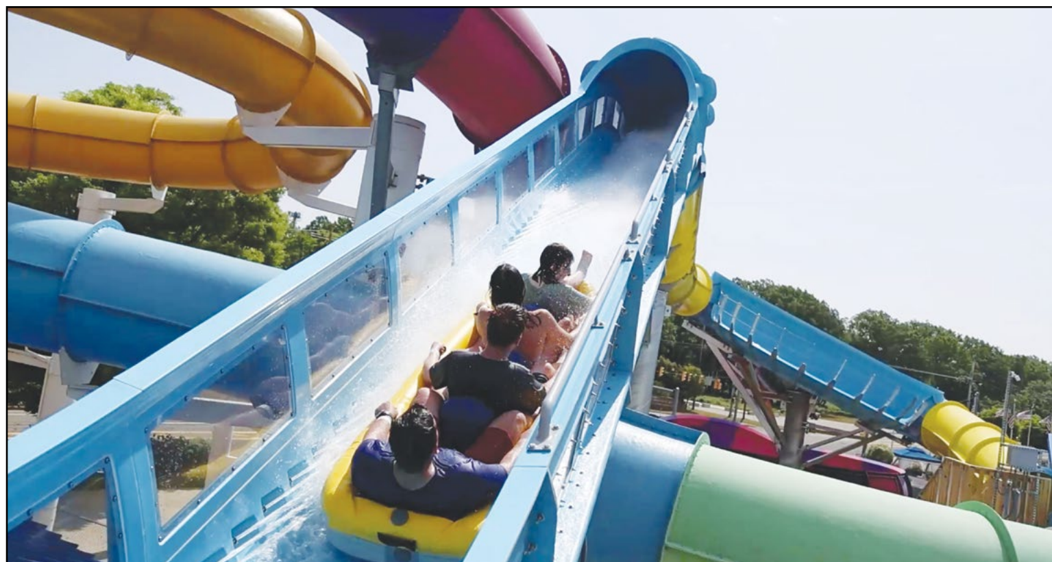
Strategically placed water jets blast rafts full of riders uphill three times throughout the ride's course. COURTESY WALDAMEER & WATER WORLD
