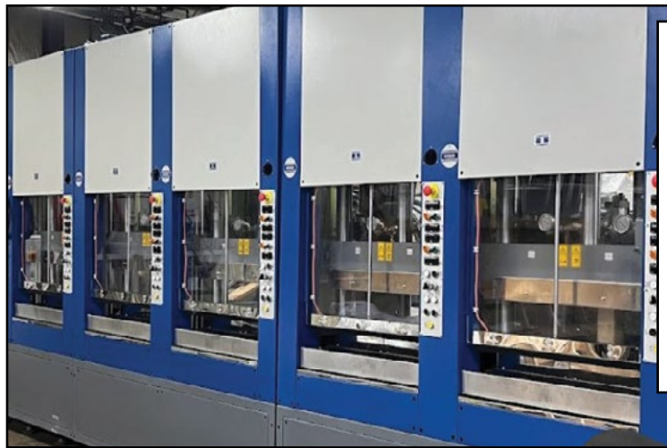
EVA is the material used to manufacture Crocs footwear and — thanks to a machine in-house at Ralph S. Alberts Co., (above) — will soon be used to make lighter and more resistant amusement ride safety padding (inset). COURTESY RALPH S. ALBERTS
