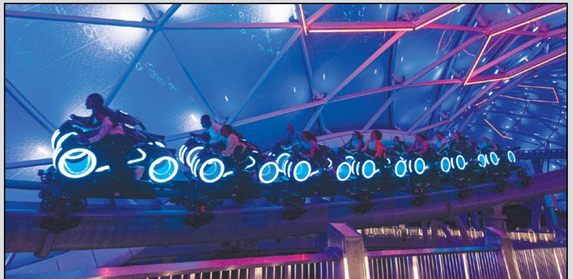
The ride utilizes a custom Vekoma Rides' Motorbike model roller coaster on which the 14 motorbikes of the coaster's seven trains have been transformed into Lightcycles.. AT/DAVID FAKE
