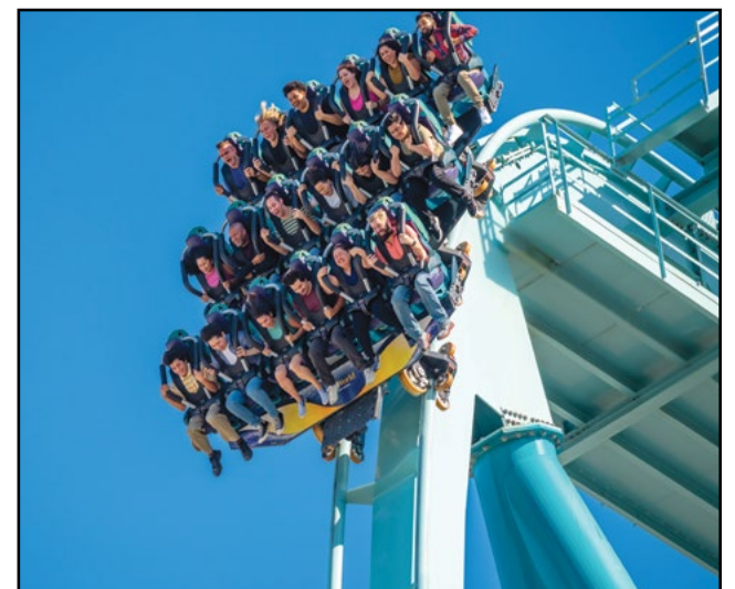
The much-anticipated new Emperor dive coaster at SeaWorld San Diego opened on March 12. Manufactured by Bolliger & Mabillard, the coaster rises 153 feet into the air and offers a 143-foot vertical drop with riders facing downward. Seating configuration for the coaster is three, six-person cars for a total of 18 riders. COURTESY SEAWORLD SAN DIEGO
