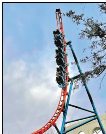
Named for the treacherous icy summits of the Arctic dessert, Ice Breaker features four airtime filled launches — two backward and two forward — one of which is a reverse launch into a 93-foot-tall spike (above middle) at a 100-degree angle, the steepest beyond vertical drop in Florida.
