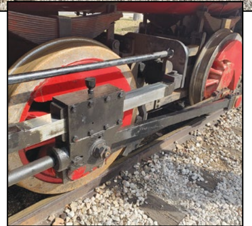
Miss Kitty (above) returned to service for the holidays and the park's 30th anniversary in 2022. Replacing wheels and bearings (inset) were essential parts of the project. COURTESY SIX FLAGS
