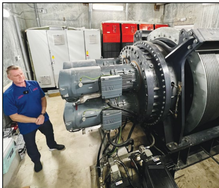
Ritchie Armstrong, owner/CEO of the Slingshot Group, gave Amusement Today an exclusive peek at the gargantuan four-ton motor and cable spool (above) that pulls the close-to-800-foot, 30mm cable that hoists the carrier car and passenger gondola to the top of the Orlando FreeFall’s tower (left).
