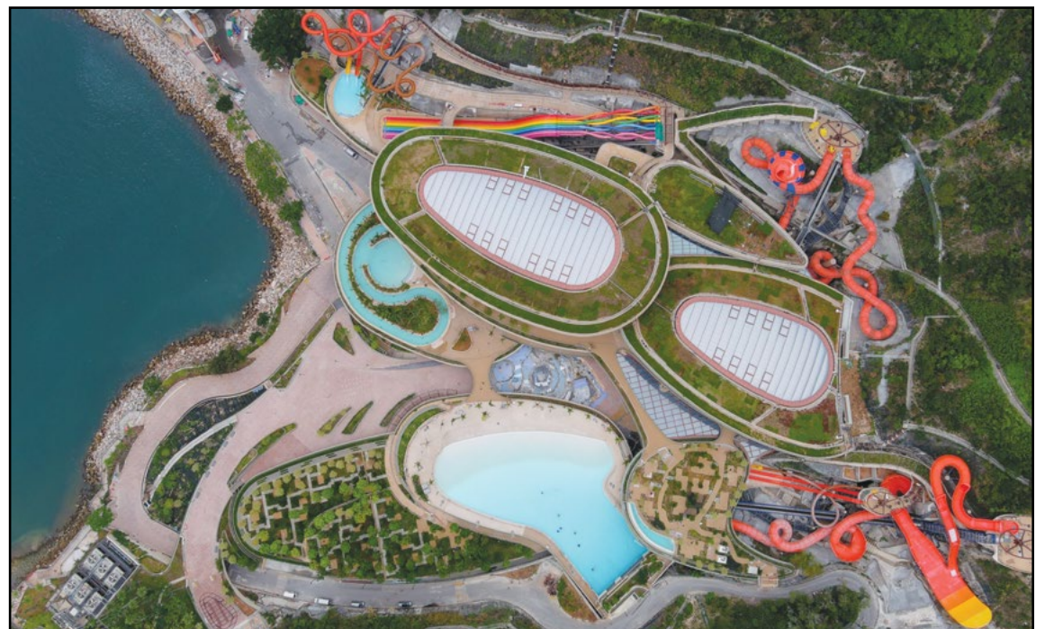
These aerial views show the massive ETF skylight system surrounded by a green roof as well as the multiple levels and careful placement of each attraction. COURTESY OCEAN PARK WATER WORLD
