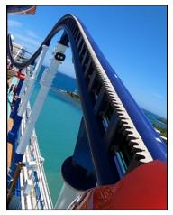
upward section or may become too fast for the next turn. That's why every Spike ride is equipped with a powerful motor and a drive wheel. In addition, a gear rack is attached along the entire track. This patented toothed system allows the electric motor drive force to be transmitted at any point on the rail, even in the tightest curves and even in vertical sections of the track."
