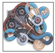
speeds up to 30 mph. On the larger, outer bowl, centrifugal force will carry the raft high onto the sides of the bowl. In the smaller inside bowl, riders should get at least two full rotations before dropping into the center. Each ride path is approximately 160 meters (525 feet). Theoretical capacity of the attraction utilizing two-person rafts is 720 riders per hour.
