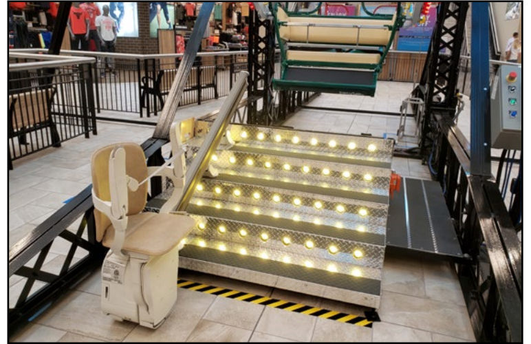
Operator Bill Peterson (above left) shows the touch-screen system that boasts operational and safety features. A lift chair and transfer system (above right) allows physically challenged riders to easily board the wheel from the loading platform. At right, Scheels showcases their business partners, both nationally and locally, by placing different logos on each basket. AT/TIM BALDWIN
