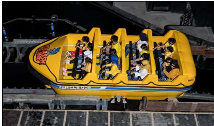
Boats move onto a moving platform and are secured to the motion base before experiencing dramatic motion during the adventurous 3D film. COURTESY JUSTIN GARVANOVIC
