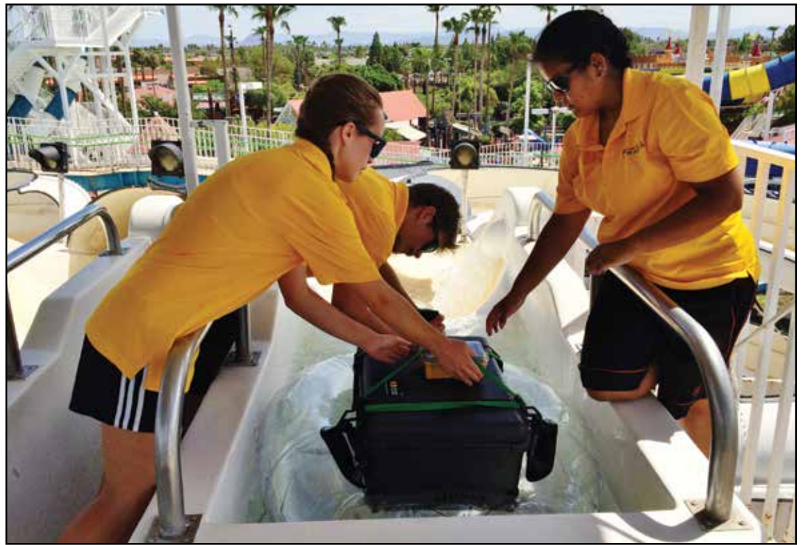
W.A.S.H.E.R. project interns Julia King, Bradley King and Joskua Carillo attach an accelerometer to the tube slide surrogate at Golfand-Sunsplash in Mesa, Ariz. COURTESY RECREATION ENGINEERING
