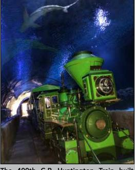
The 400th C.P. Huntington Train built by Chance Rides replaces the gasoline-powered engine with an electric one that runs on lithium-ion batteries. The train's color reflects its newfound environmental friendliness.
